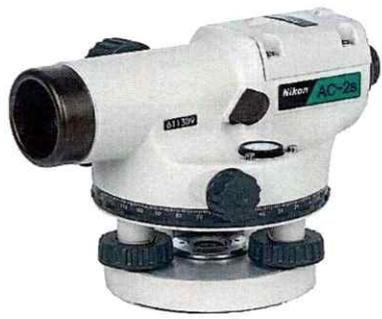
A precision level with a white and black body. It has a large objective lens on the left and is labeled "Nikon AC-28".              |
